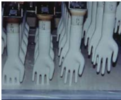
Image 1. Glove formers being dipped into the liquid glove solution.
