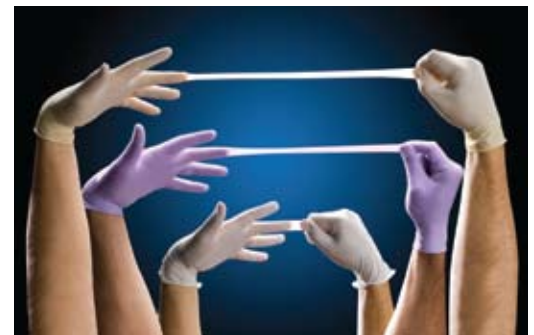
Image 2. Three types of base glove materials (from top): natural rubber latex (NRL), acrylonitrile-butadiene (nitrile) and polyvinyl chloride (vinyl, PVC).
